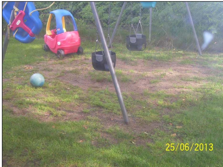
**Photograph 6: No protective material (mulch or wood chips) under a swing area.**
