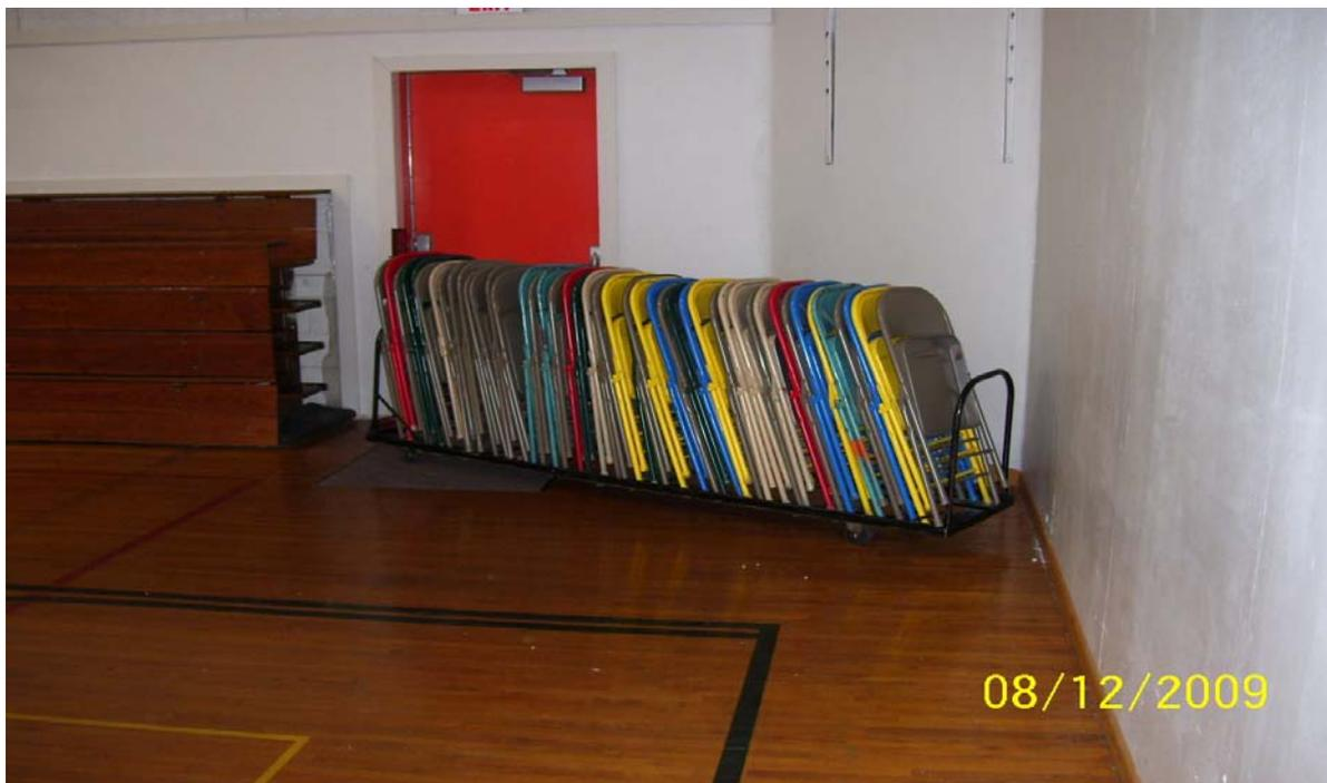
**Photograph 2 – Taken at North Fond du Lac on December 8, 2009, showing a rack of folding chairs blocking an exit.**
